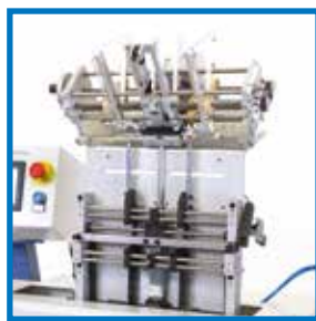
Hangers-forming and feeder for 100-300 mm. hangers.
